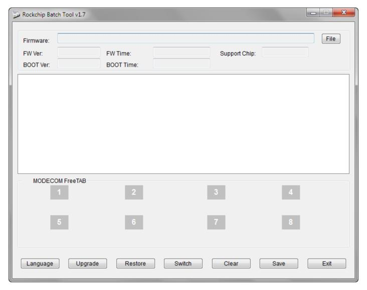
5. Turn off the tablet and connect it to the computer using usb cable, then **press and hold VOL+** button, next press the **Reset** button and keep still about 5 seconds down the **VOL+**, tablet will be detected by the system (the drivers will not be added automatically by the system, please follow the description which is below the photo)
