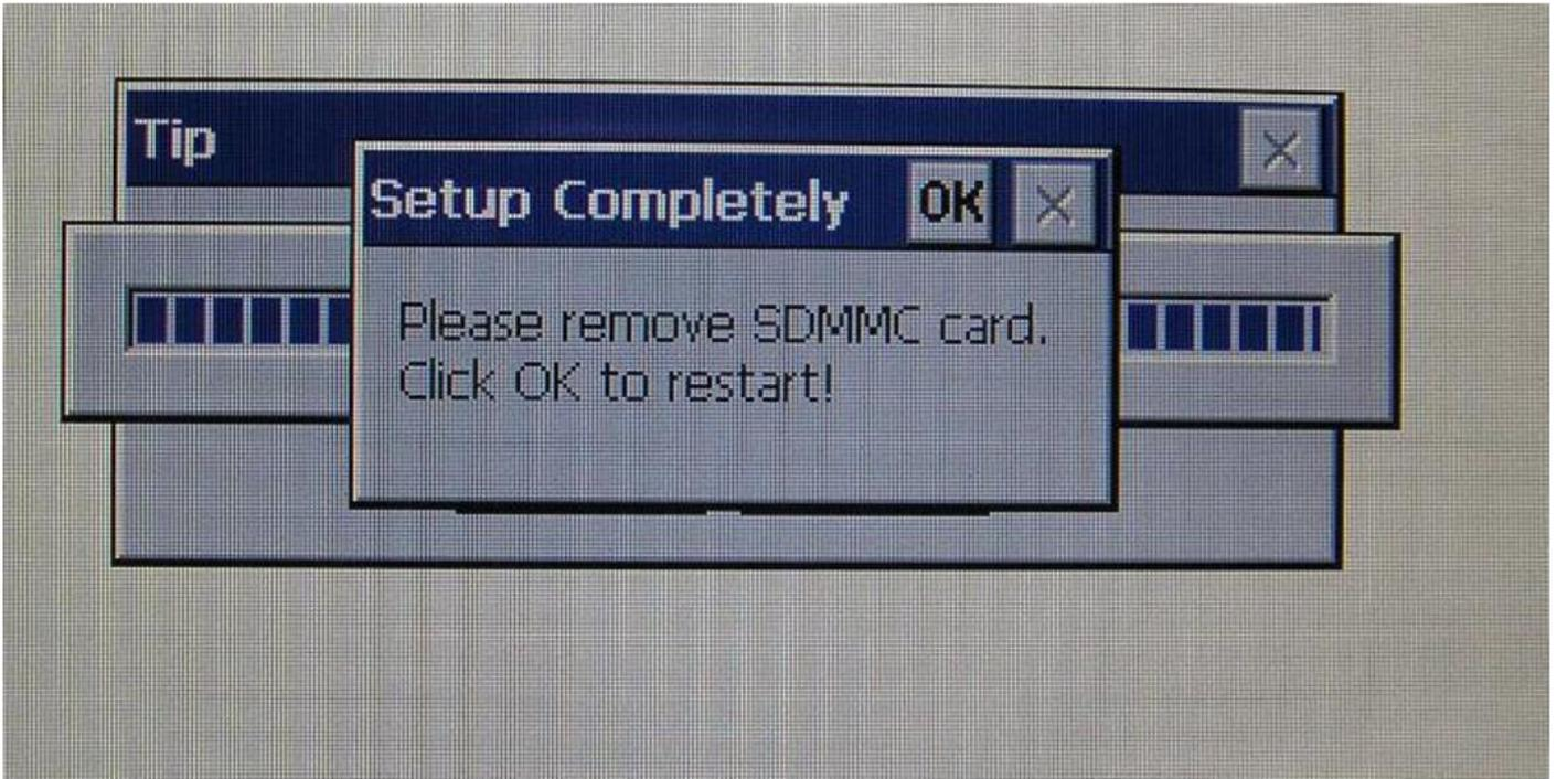
7. Remove the microSD card from the device and confirm > **OK**, then delete the files from the card
