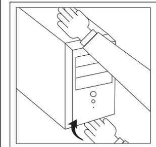
Please take hold top side of chassis using one hand and pull out the bottom side of front panel using another hand
