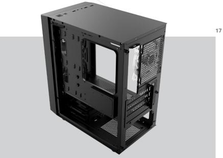
The installation of HDD or SSD drives is of course also well thought out here. Inside the case in a tunel there is a basket for  $2 \times 3.5$ " or 2.5" drives.
