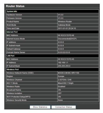
This page displays the information of the current running status of the device, including system information, connection status of the Internet port, LAN port, and wireless port, and traffic statistics of each port.
