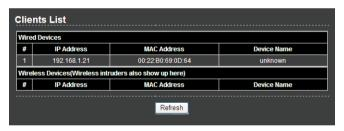
This page displays the information of computers connected to the router, including the IP adress, device name, and MAC address of each computer.
