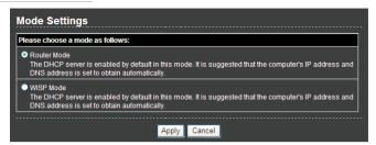
In router mode, the device works as a router. WDS function is supplied to expand wireless network. If WDS function is enabled, the device could work as a "Wireless Repeater" and communicate with another "Base Station mode" wireless device to expand the "Base Station", or it could work as a "Wireless Base Station" and communicate with another "Repeater-mode" wireless device to expand the "Repeater".
