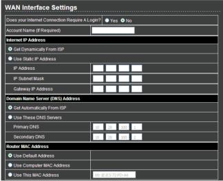
The router supports 3 modes of WAN connection: Dynamic IP (DHCP), Static IP (Fixed) and PPPoE. In this page, you can select an appropriate WAN connection and configure the relevant parameters according to the actual requirements.
