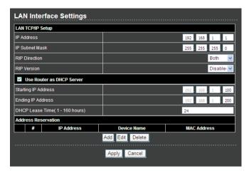
In this page, you can configure the parameters of the LAN port. You can modify the IP address of the LAN port according to the actual network environment.
