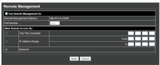
The remote management function allows you to configure the router in the WAN through the Web browser. In this way, you can manage the router from a remote host.
