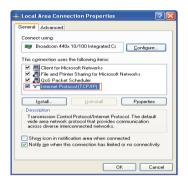
Step 7 Set the IP address of your computer to 192.168.1.X (X is an integer in the range of 2 to 254), and the MAC address to 255.255.255.0. Set the gateway and the IP address of the DNS server. You can leave them blank if you do not know information about the gateway and DNS server. Click OK.
