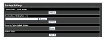
In this page, you can export the configuration information of the router in a file to the computer for later use, import a previously saved or a new configuration file, restore the factory default settings of the router, and reboot the router.
