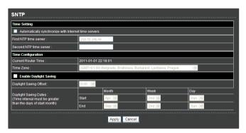
In this page, you can set the time information of your router. It is strongly recommended to set the correct time on the router first. This ensures proper functioning of log, site blocking, and schedule, because these functions are based on the time setting in this page.
