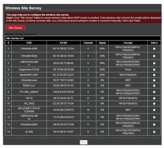
Configure the device manually so it has the same wireless security settings as the wireless modem network which you selected, then device can communicate with the selected network.
