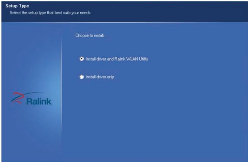
NOTE: you may select the second method when you are accustomed to use the WINDOWS built-in wireless configuration program. However, this program doesn't support AP mode, WPS, and the WPS button on the wireless adapter. To use these advanced features, the first method is recommended.
