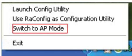
In this mode, the wireless adapter acts as an AP to transmit wireless signal and create a wireless network, while allowing other wireless clients to access this network.
