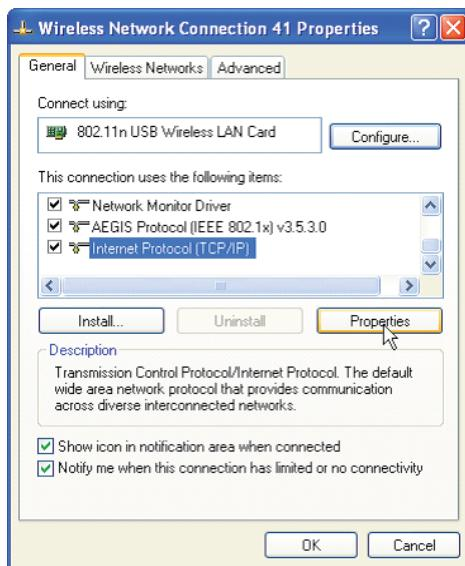
Please enter the IP address and subnet mask, and make sure this IP address is not used by other devices in the network. For example: if your wireless adapter's IP address is 192.168.0.1, then set other wireless adapters' IP addresses within the range of 192.168.0.2—192.168.0.254. Click "Ok" to save the settings.
