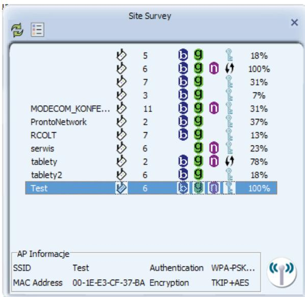
For the networks that are not encrypted, you can directly click "Connect". However, for the encrypted wireless networks, a "Profile Settings" dialog will pop up and you must select the corresponding authentication type and encryption type, and then click the "Next" button to input the correct key. Please note that this type of connection will not create a profile, thus next time connect to this network you still need to select it manually.
