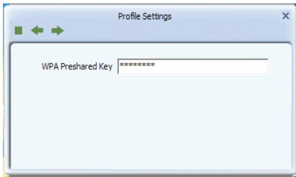
After a profile is successfully added, the profile can be seen on the profile list, select it and click the "Active" icon on the lower right corner. And then search for the wireless network on other clients. Double click the wireless network you have configured and you'll be prompted for the key .After entering the key, click "Connect".
