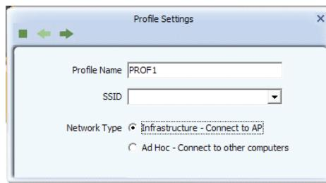
Infrastructure is an application mode that integrates the wired and wireless LAN architectures. It is different from Ad-Hoc in that in this mode the computer installed with the wireless network adapter has to fulfill the wireless communication via AP or wireless router. It can be divided into two modes: "wireless AP + wireless network adapter" and "wireless router + wireless network adapter".
