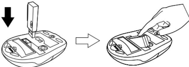
When the receiver is in the compartment of the mouse, power supply is automatically off to stop power consumption.
